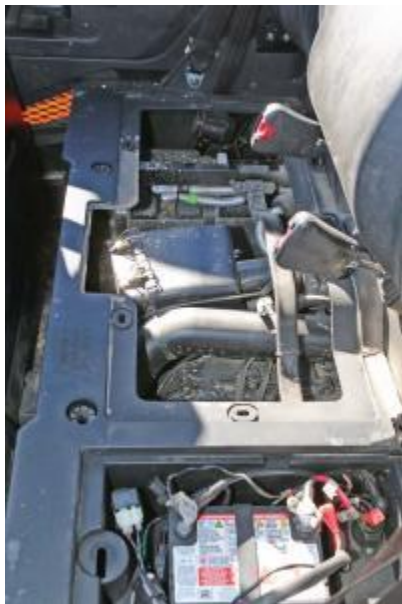
Under the seat of the Challenger 550 and Challenger 750 is the battery, and easy access to the airbox.
