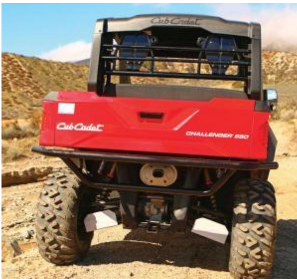
The rear of the Challenger 550 and 750. Notice the 2" receiver hitch (on the front as well), the center mounted exhaust, and standard lower A-arm guards.
