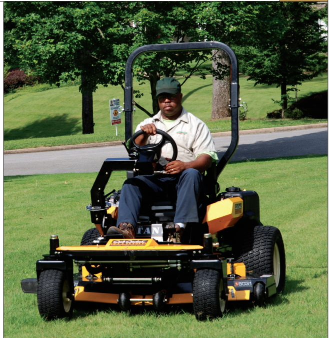
A pivoting front axle on the Tank S helps provide a uniform cut even when the terrain is slightly uneven.
