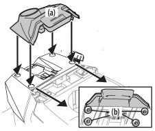
**NOTE:** Be sure to press on the lower part of the dash cap (a) facing the operator position to ensure the lower tabs on the dash cap are in place.
