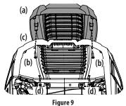
4. Tighten all four screws to 16-24 in-lbs (1.8-2.7 N-m).
