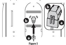
**NOTE:** The tractor will not operate without the seat switch wiring harness connected.
