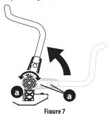
If the lapbars do not line up after making the knob adjustment, loosen nuts (b), align lapbars and retighten nuts.
