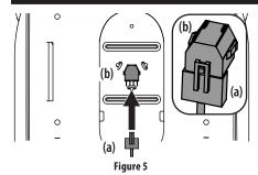
**NOTE:** Tractor will not operate without the seat switch wiring harness connected.
