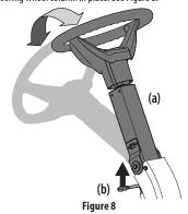
**NOTE:** When the steering column adjustment lever is lifted, the steering wheel column will begin to raise up. Apply downward pressure on the steering wheel to lower the steering wheel column, if needed.
